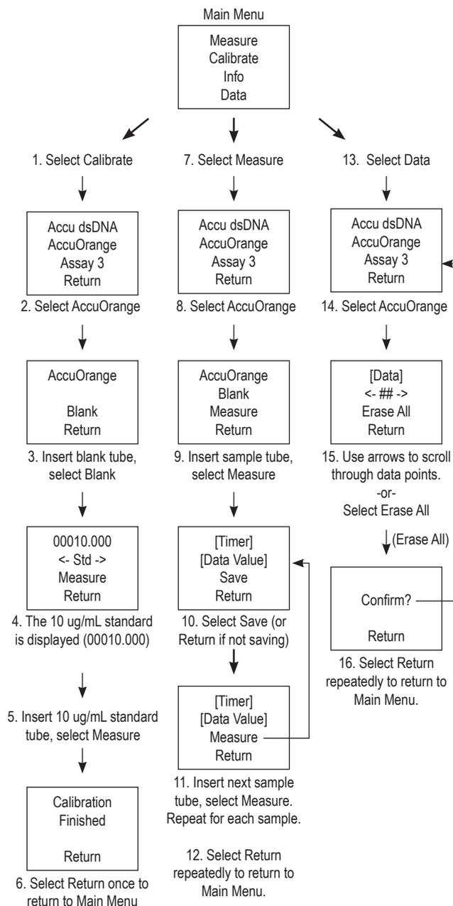
Figure 4. AccuLite user menu tree showing AccuOrange calibration, measurement, and data retrieval steps. See the AccuLite user manual for complete user menu tree.
